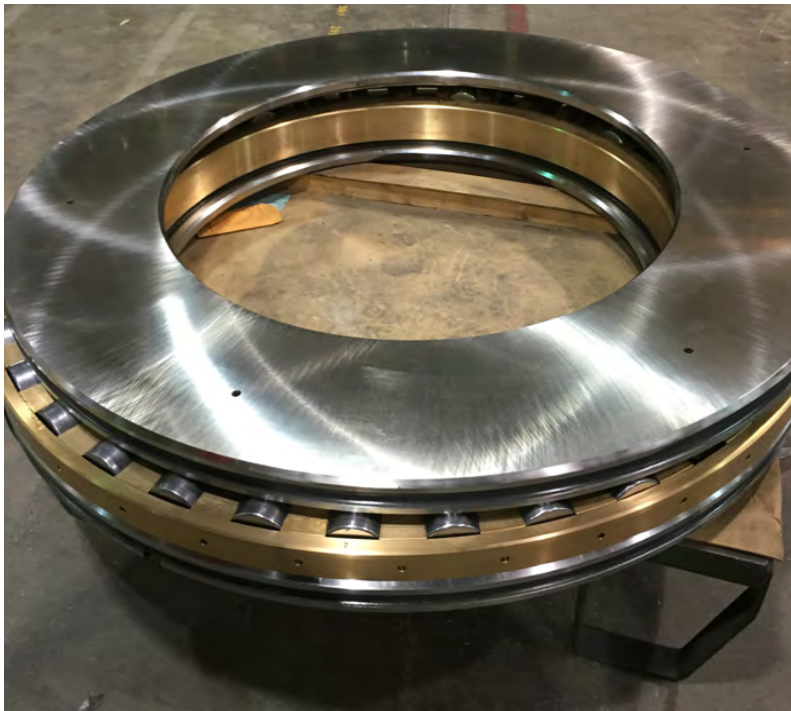
CYLINDRICAL THRUST BEARINGS LIKE THE MPS-89 BEARING ARE USED IN COAL PULVERIZERS
