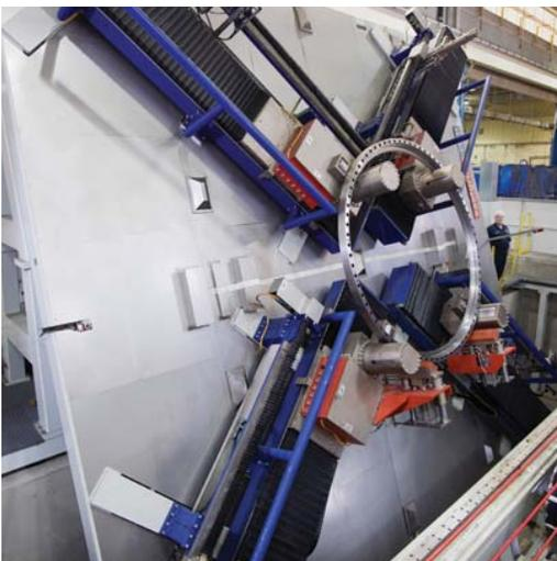
**MESSINGER INDUCTION HEAT TREATING EQUIPMENT HANDLES BEARINGS UP TO 25 FT IN DIAMETER AND 30,000 LBS TO ENSURE PRECISE BEARING HARDNESS.**
